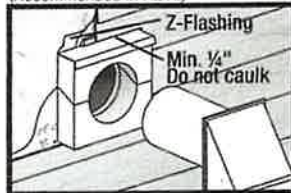
Figure 13 Block Penetration (Recommended in HZ10)
