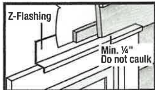
Figure 8 Ground to Siding
