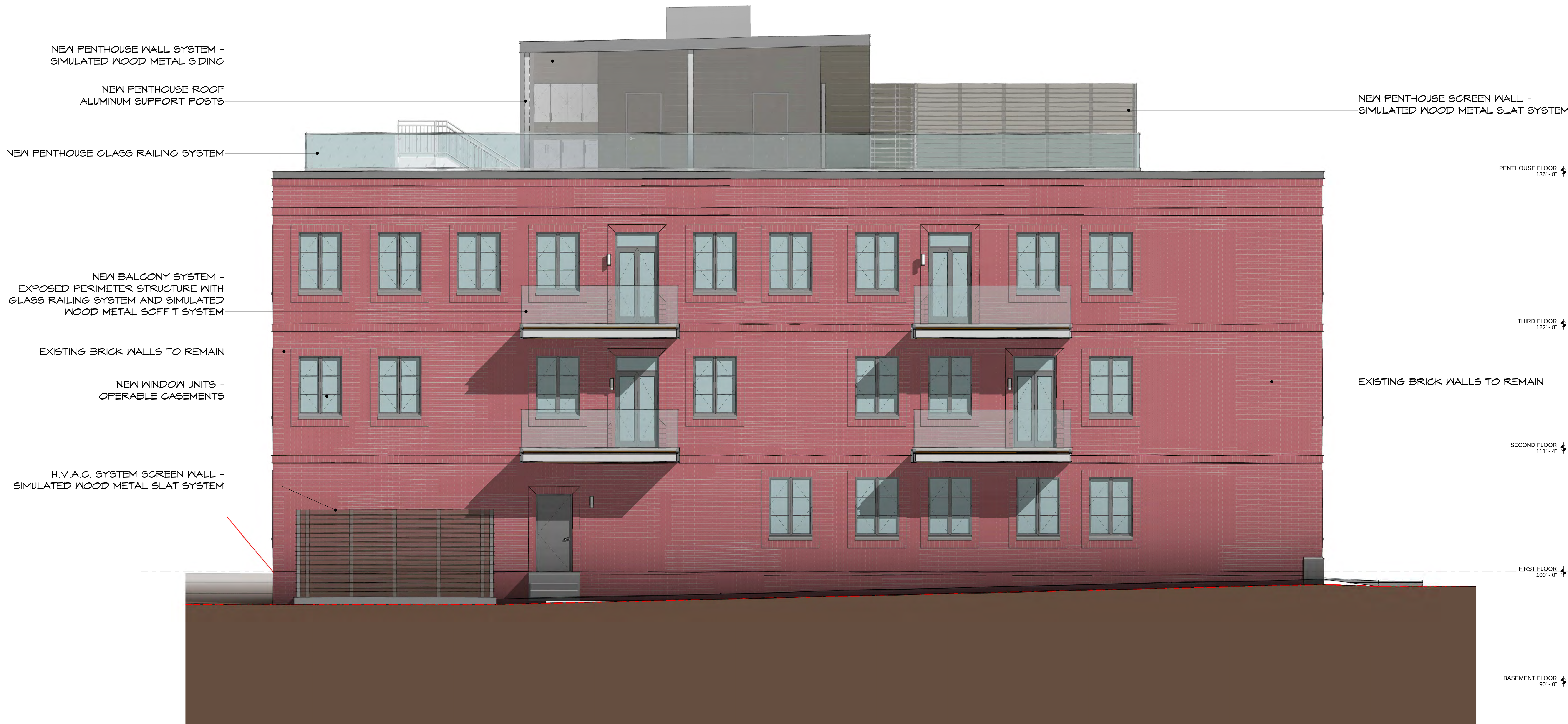
1 SOUTH BUILDING ELEVATION X5.1 1/4" = 1'-0"
