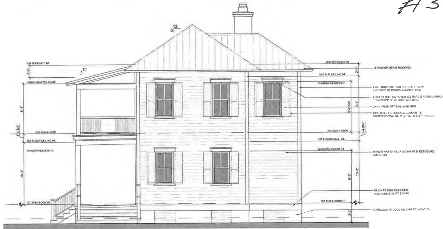
1 ENTRY ELEVATION (South) 1/4" = 1'-0"
