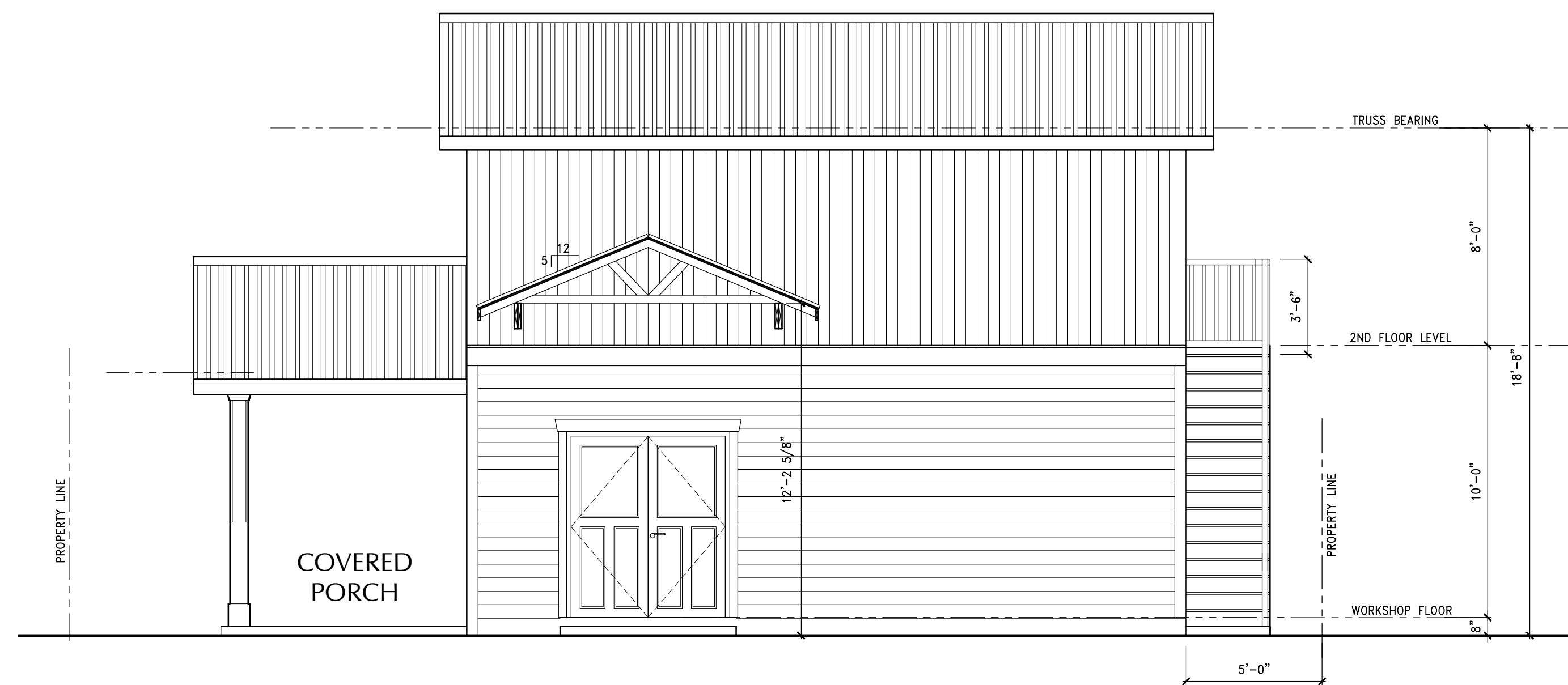
FRONT ELEVATION - SHOP/STORAGE Scale: 1/4" = 1'-0"
