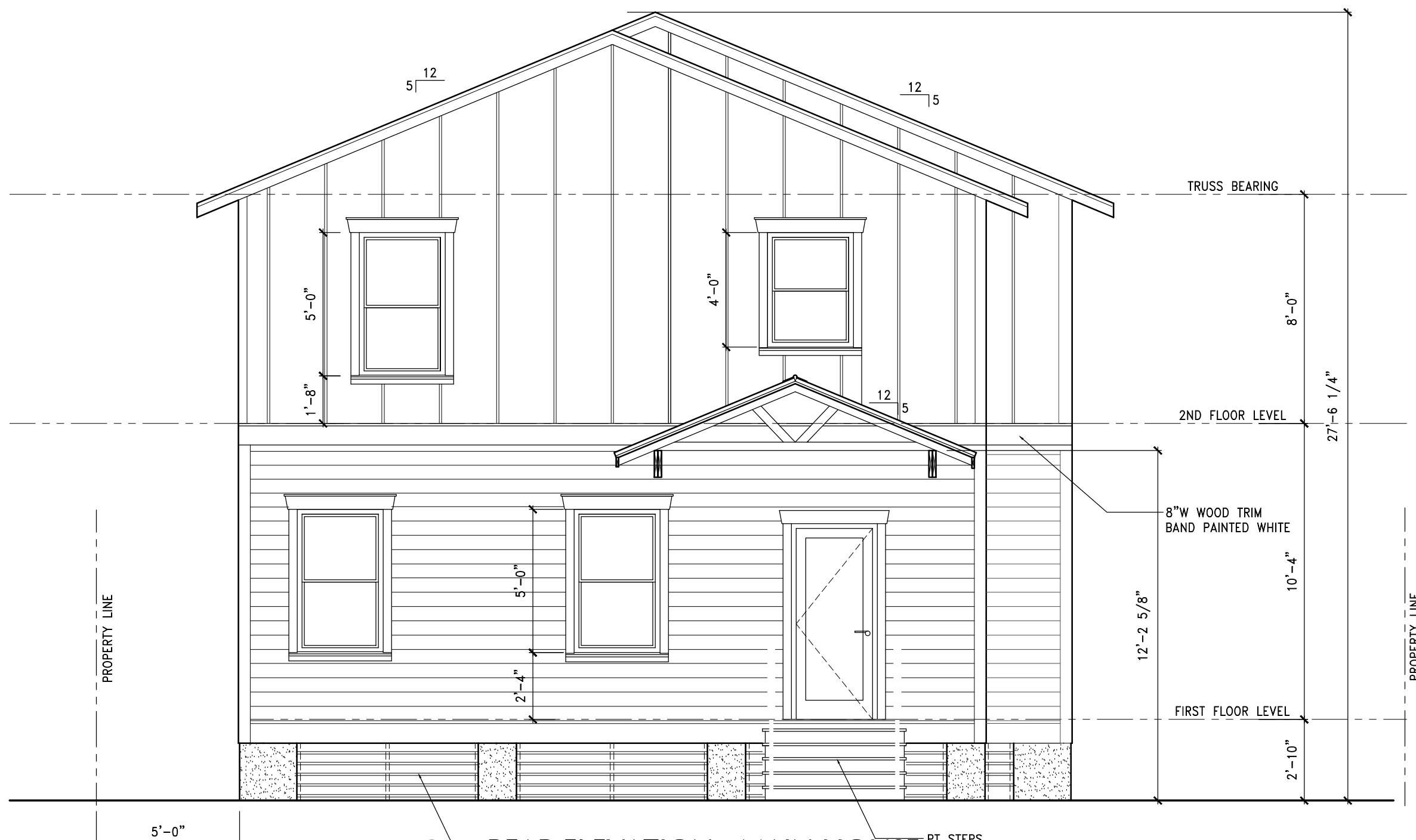
REAR ELEVATION - MAIN HOUSE Scale: 1/4" = 1'-0"
