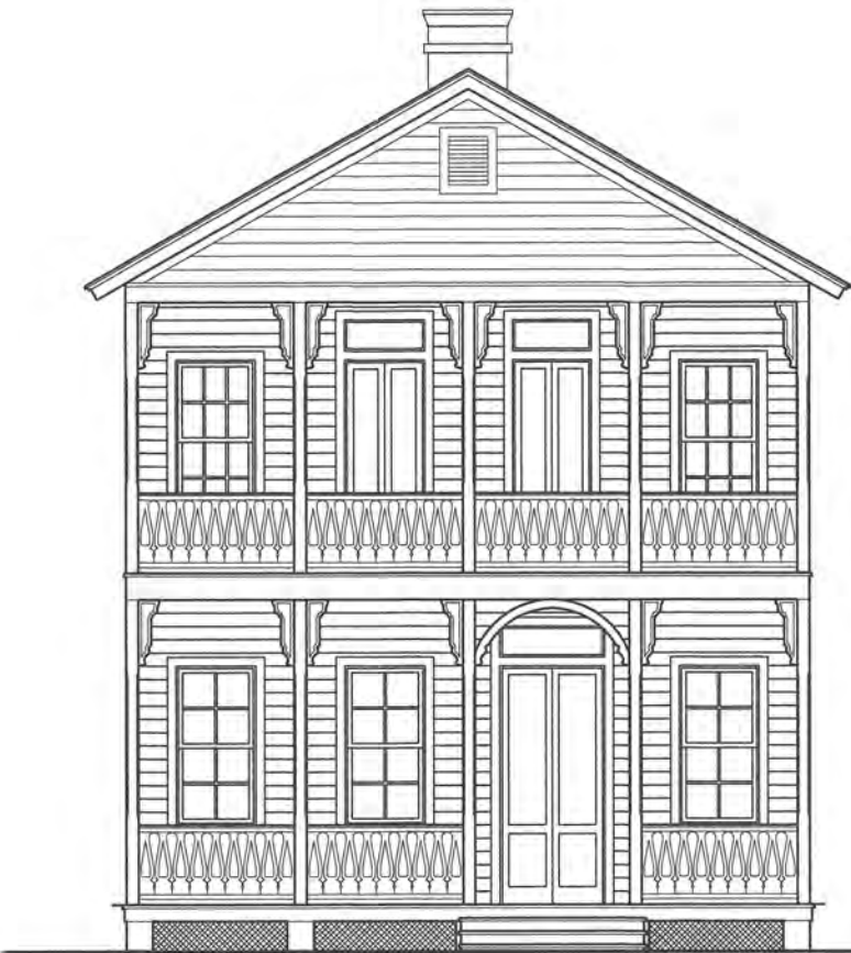
EAST A-1.2 EXISTING EAST ELEVATION 1/4" = 1'-0"
