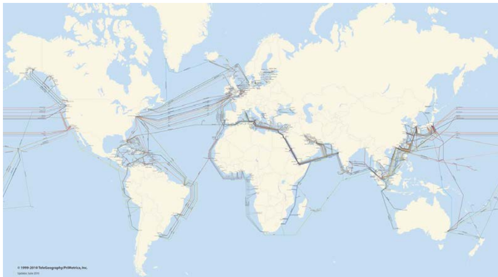
Figure 3.4-2. Submarine Cable Systems, 2010
