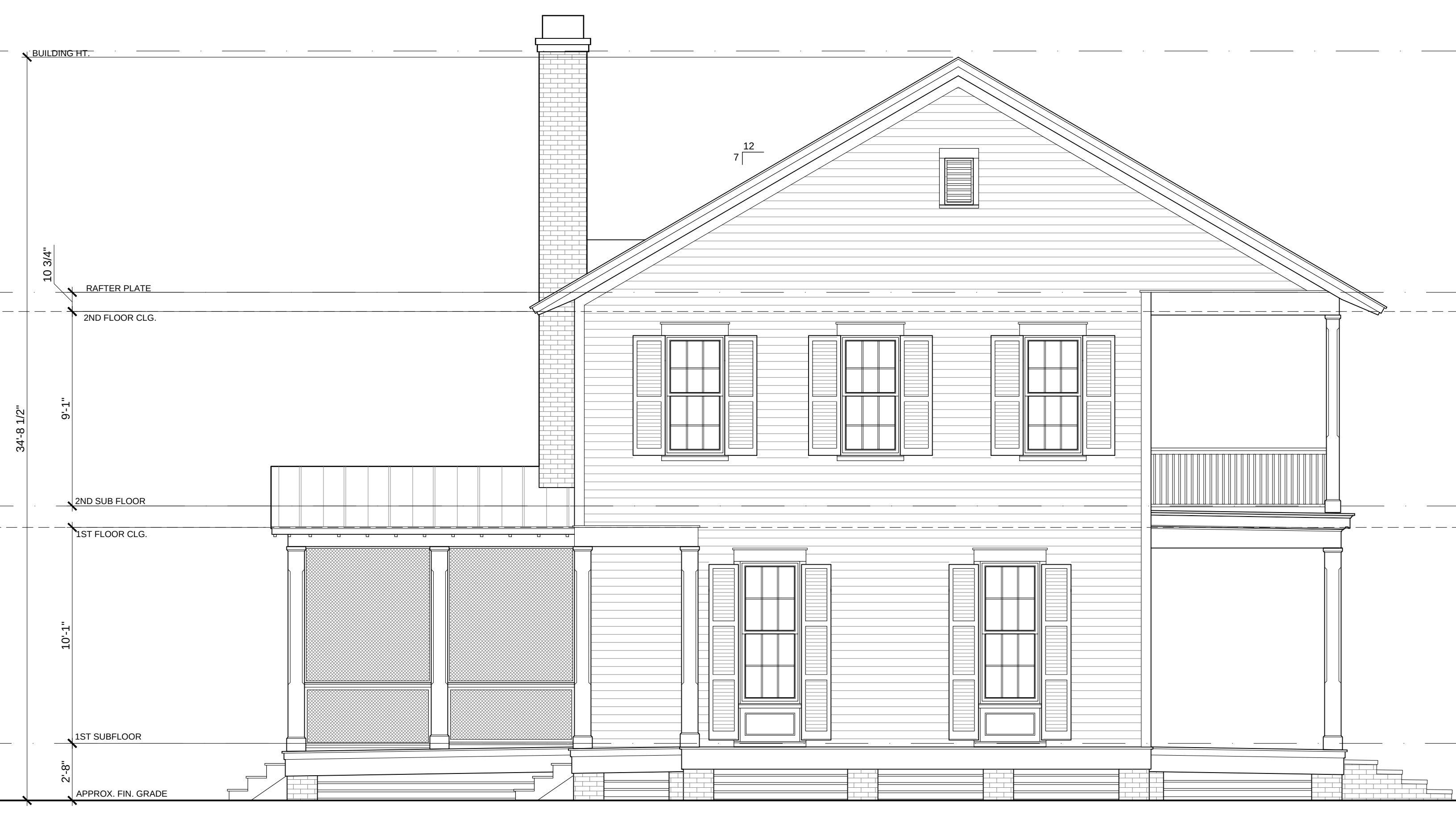
4 3 LEFT SIDE ELEVATION 1/4" = 1'-0"
