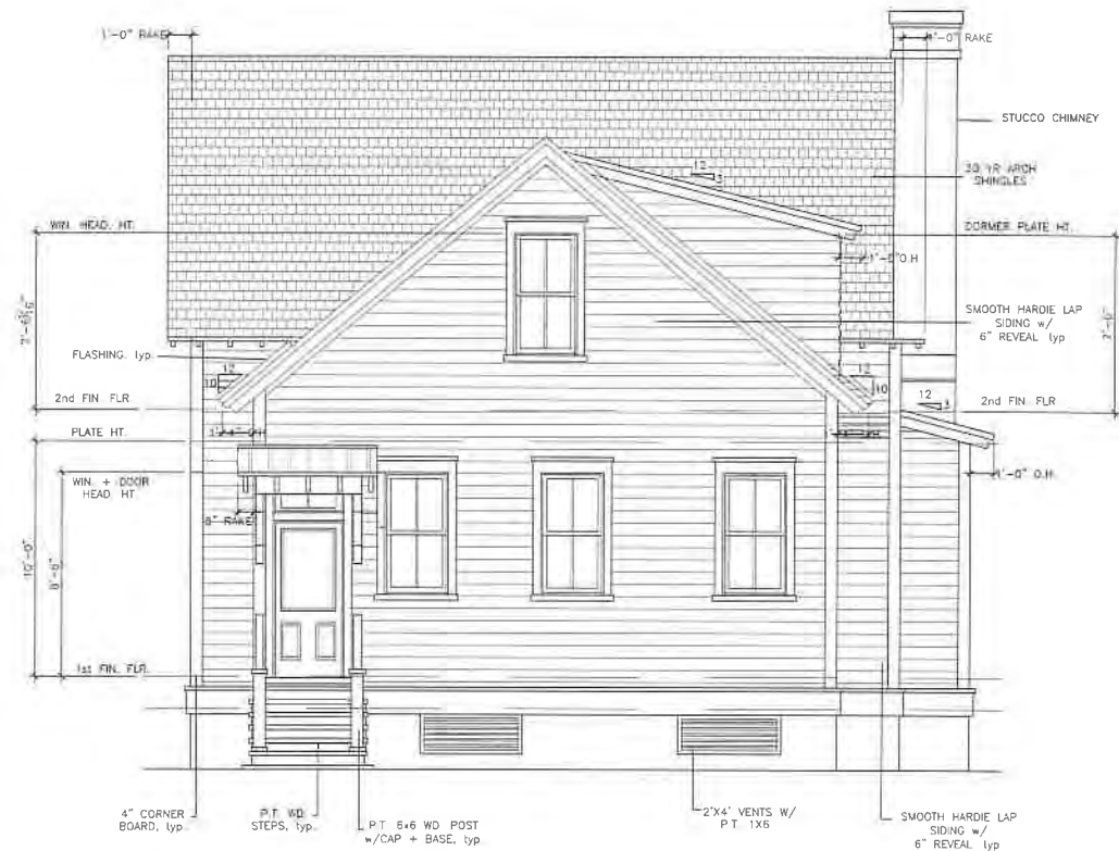
REAR ELEVATION SCALE: 1/4" = 1'-0"
