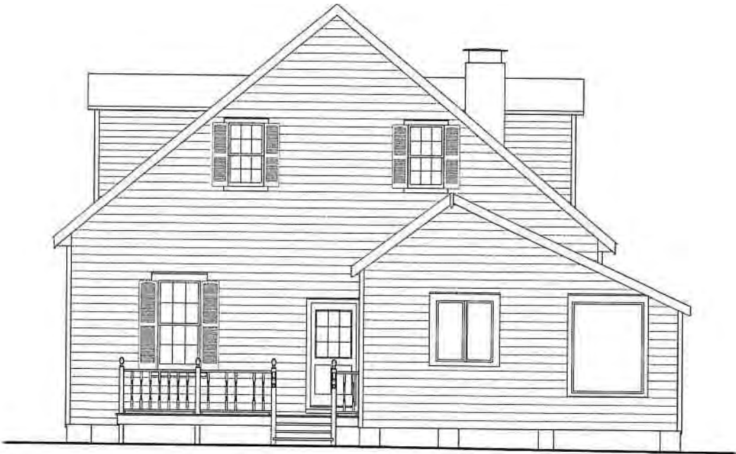
AS-BUILT EAST ELEVATION 1/4"=1'-0"
