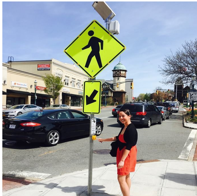
SOLAR POWERED PEDESTRIAN ACTIVATED CROSSWALK
