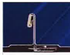
Maxima ADV & Maxima 1.5" 180° Fold
