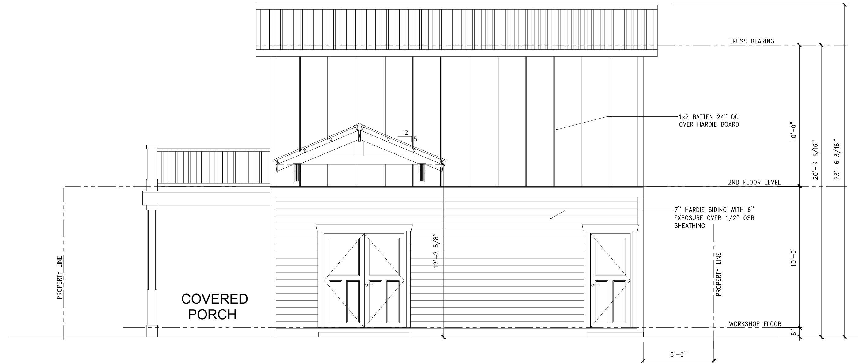
FRONT ELEVATION - SHOP/STORAGE Scale: 1/4" = 1'-0"
