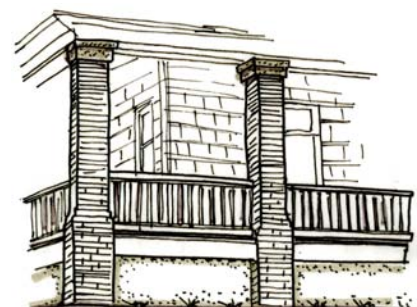
Brick Piers with Wood Railings
