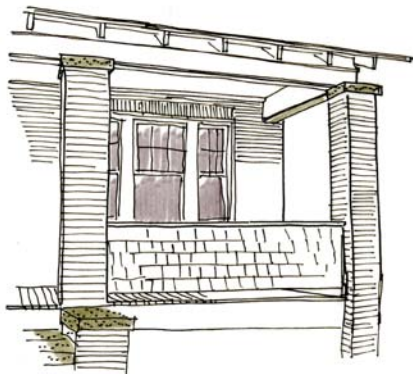
Brick Piers with Concrete Capping and Shingle Panel Railing
