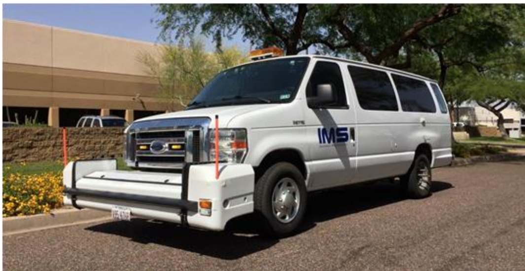
Figure 4 – Laser Road Surface Tester (RST)
