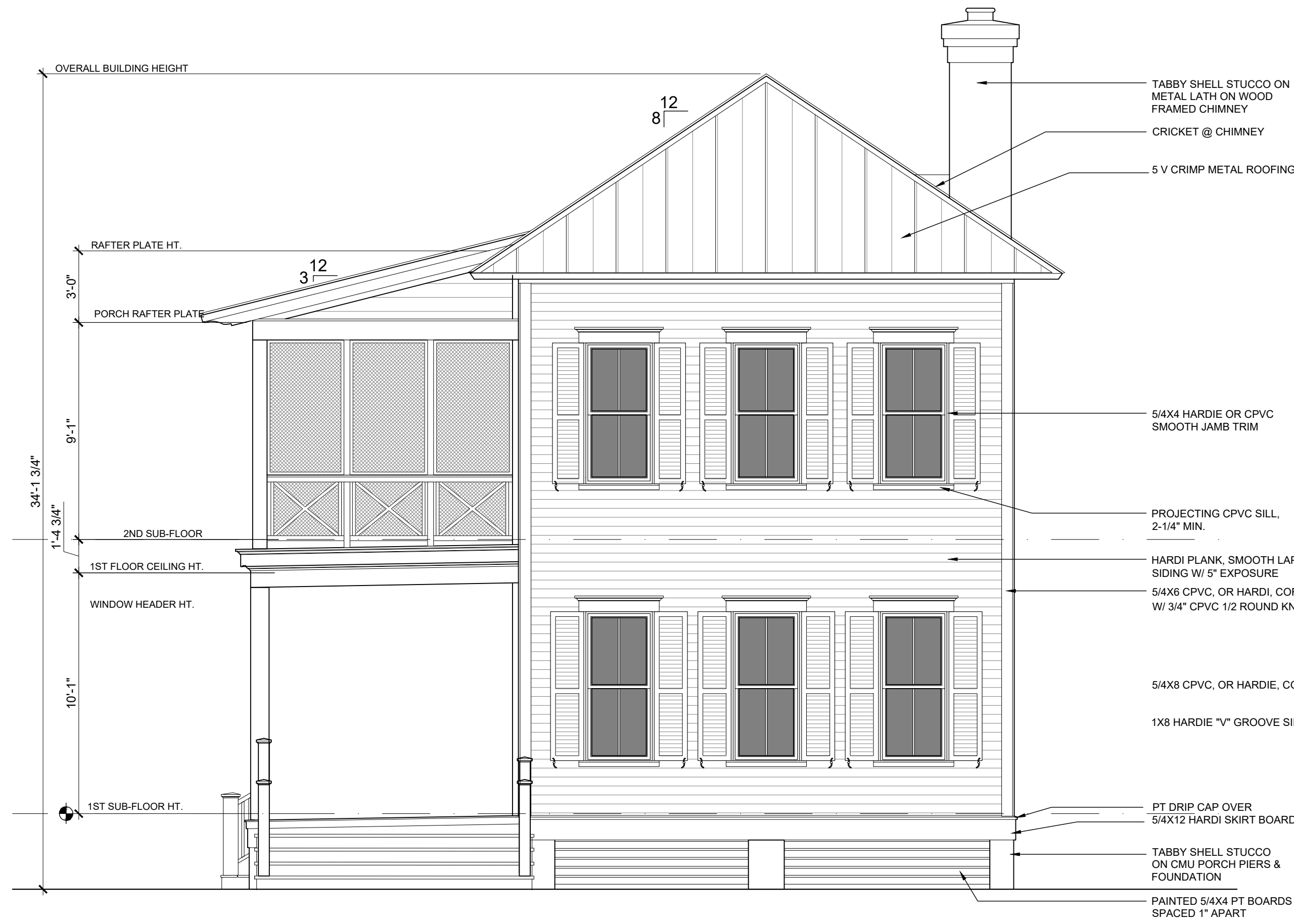
1 ENTRY ELEVATION A2.0 1/4" = 1'-0"
