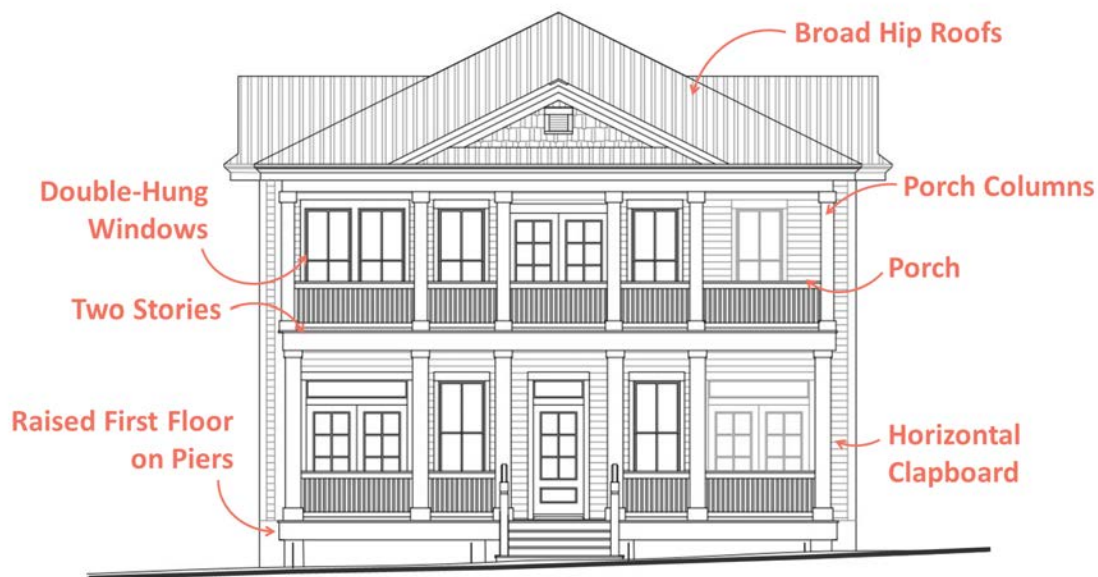
Figure 25: Low Country / Southeast Atlantic Coastal Architectural Style.
