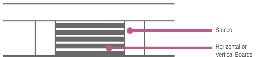
Figure 29: Example of stucco piers with horizontal wood boards in between type foundation.
