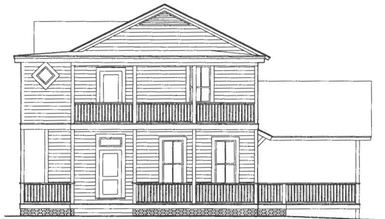
EXIST A-2.1 1/4" = 1'-0" EXISTING WEST ELEVATION
