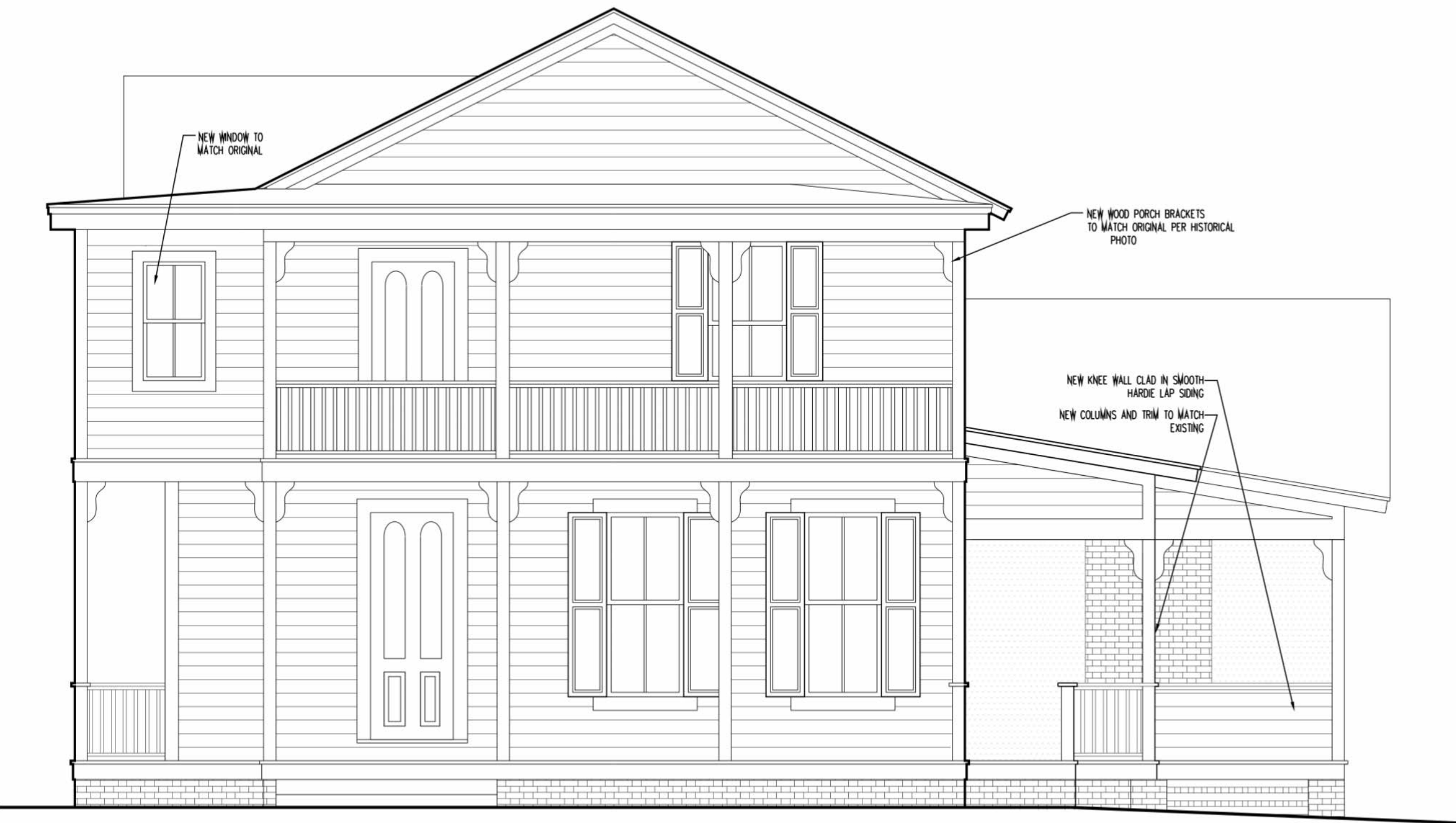
ELEV A-2.2 PROPOSED WEST ELEVATION 1/4" = 1' - 0"
