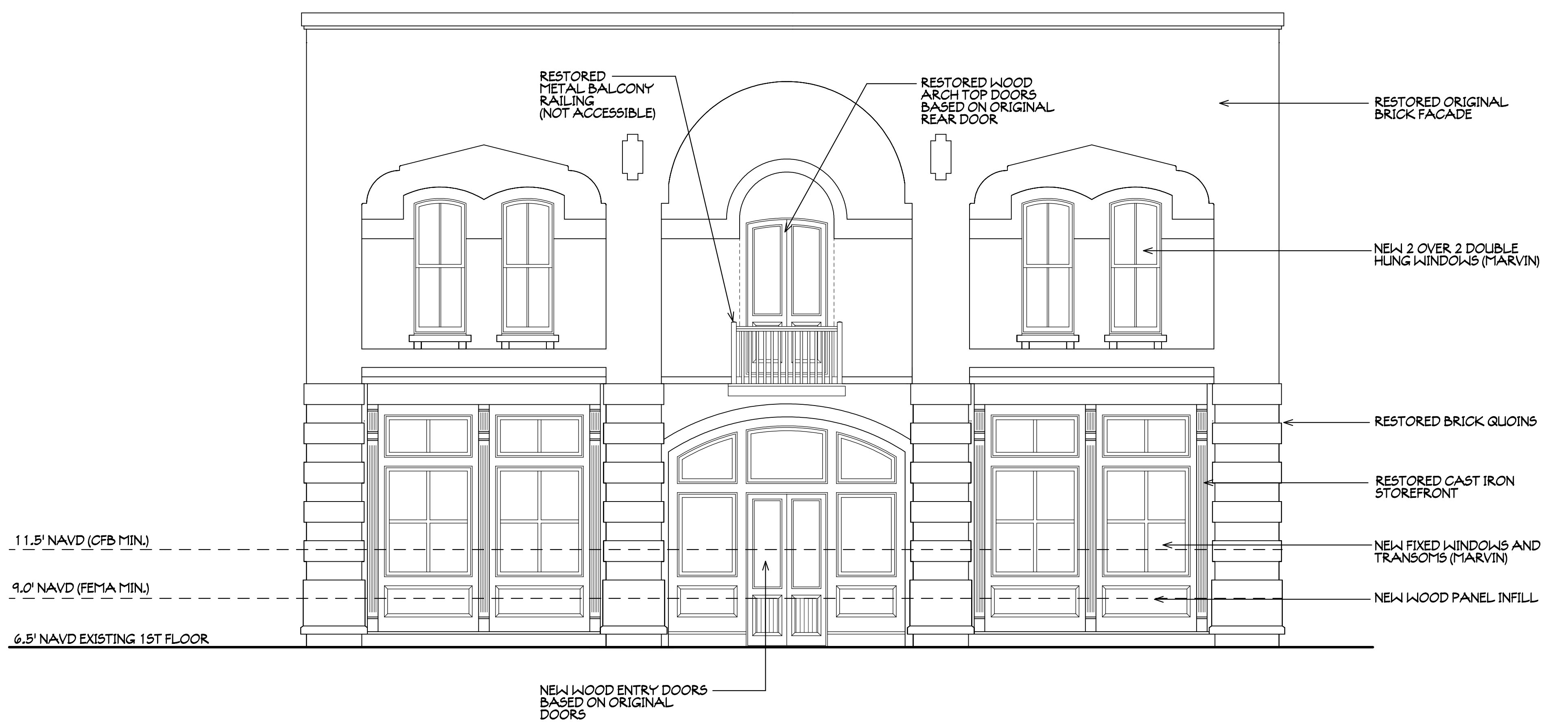
PROPOSED SOUTH ELEVATION (CENTRE STREET)
