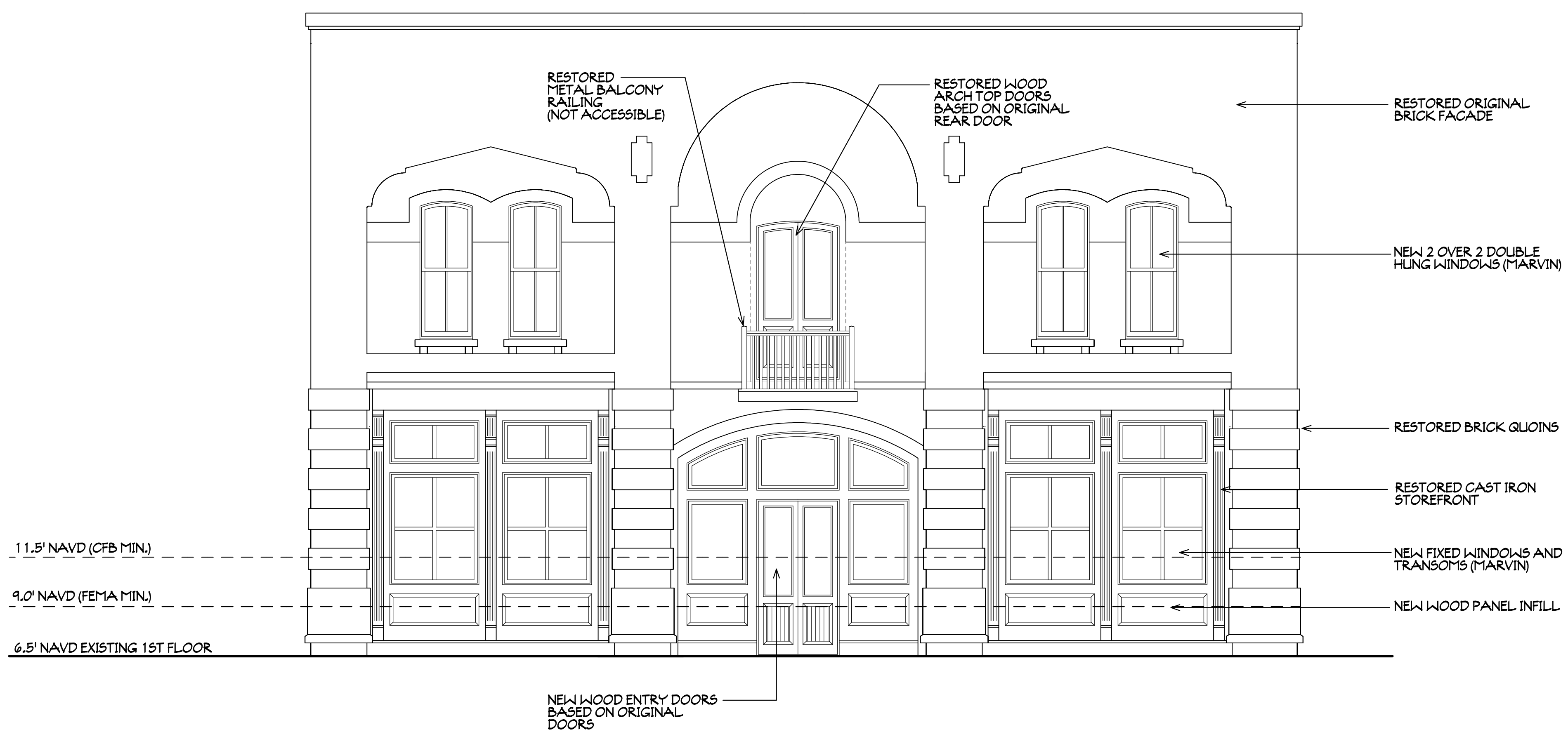
PROPOSED SOUTH ELEVATION (CENTRE STREET)
