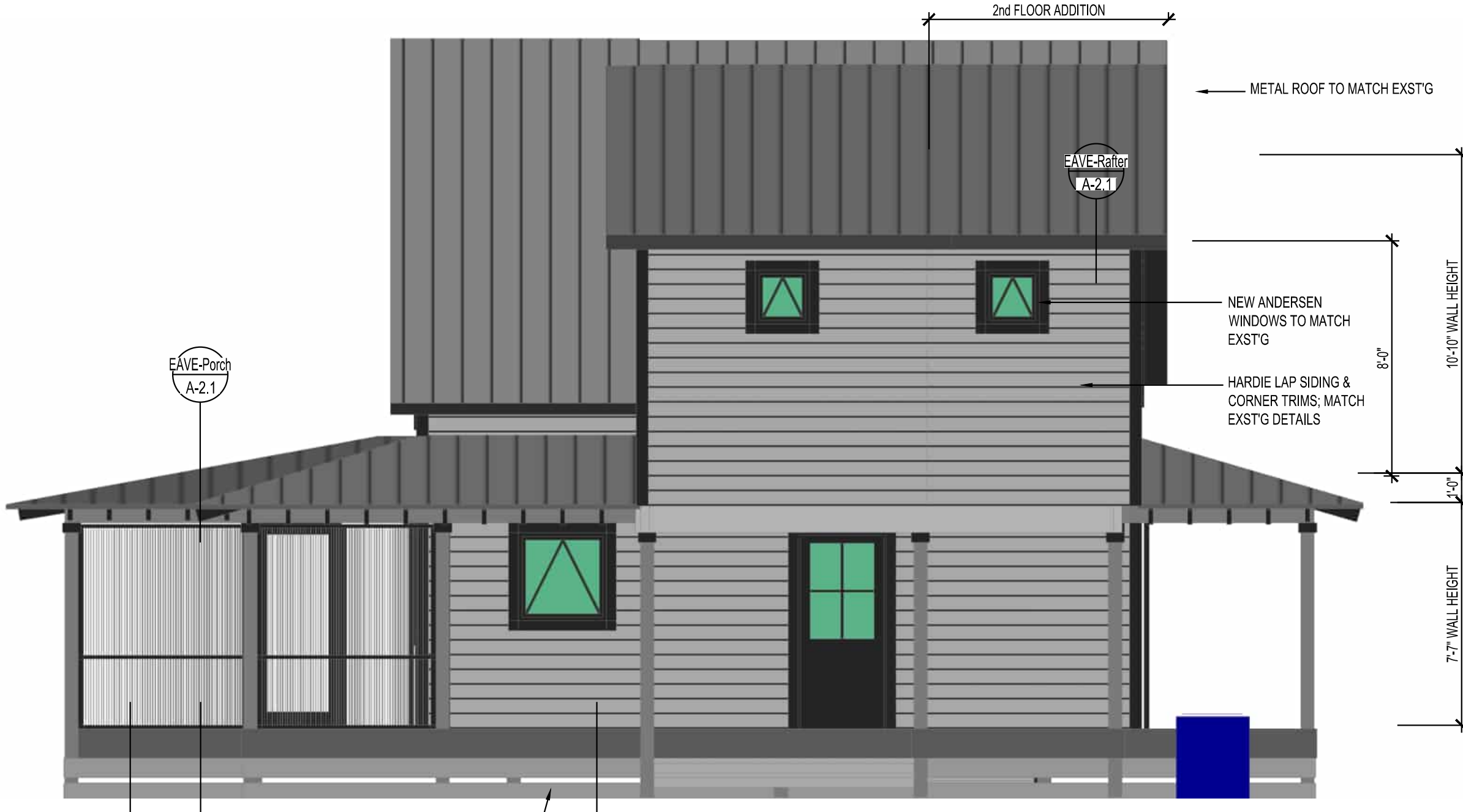
NEW NORTH ELEVATION 1/4"=1'
