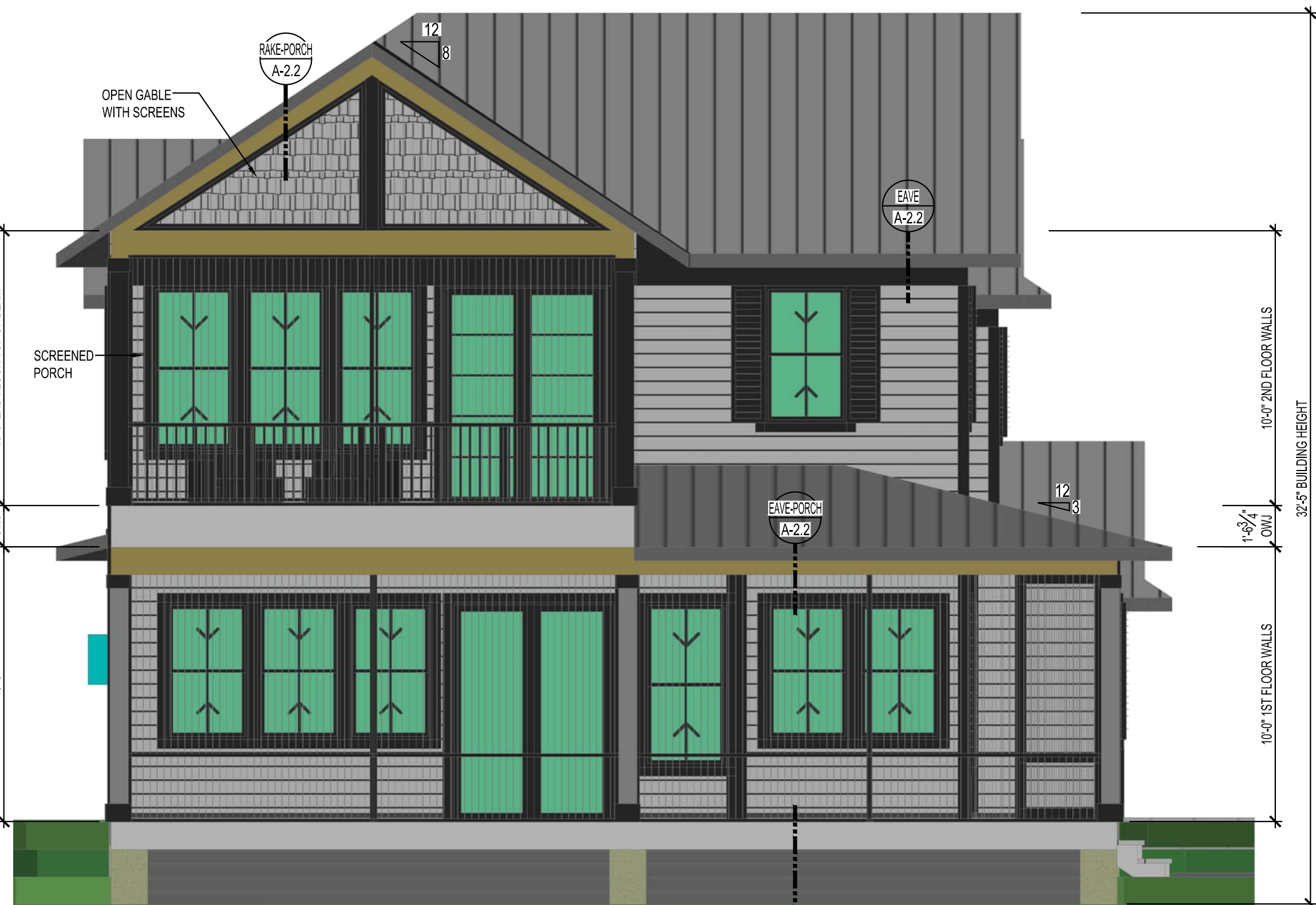
HOUSE SOUTH ELEVATION 1/4"=1'
