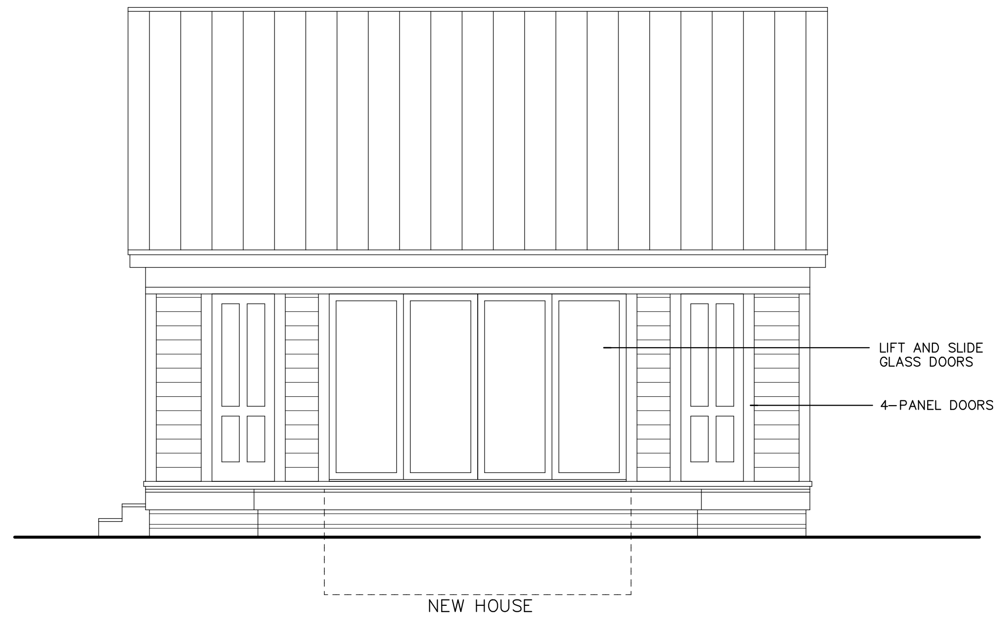
EAST ELEVATION -- MAIN HOUSE
