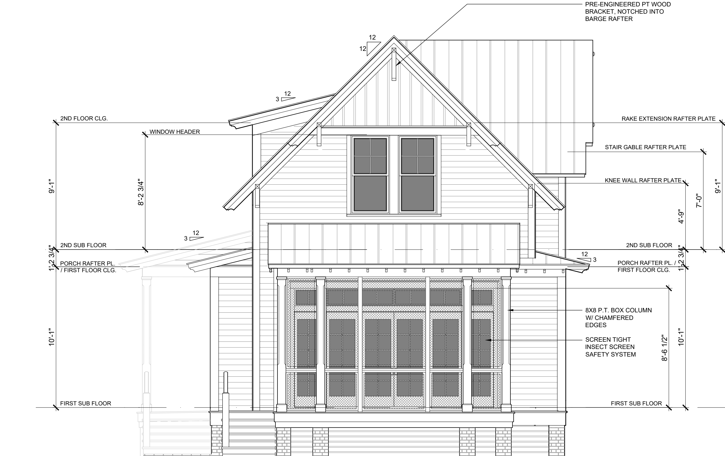
3 COURTYARD ELEVATION (SOUTH ELEVATION) 1/4" = 1'-0"
