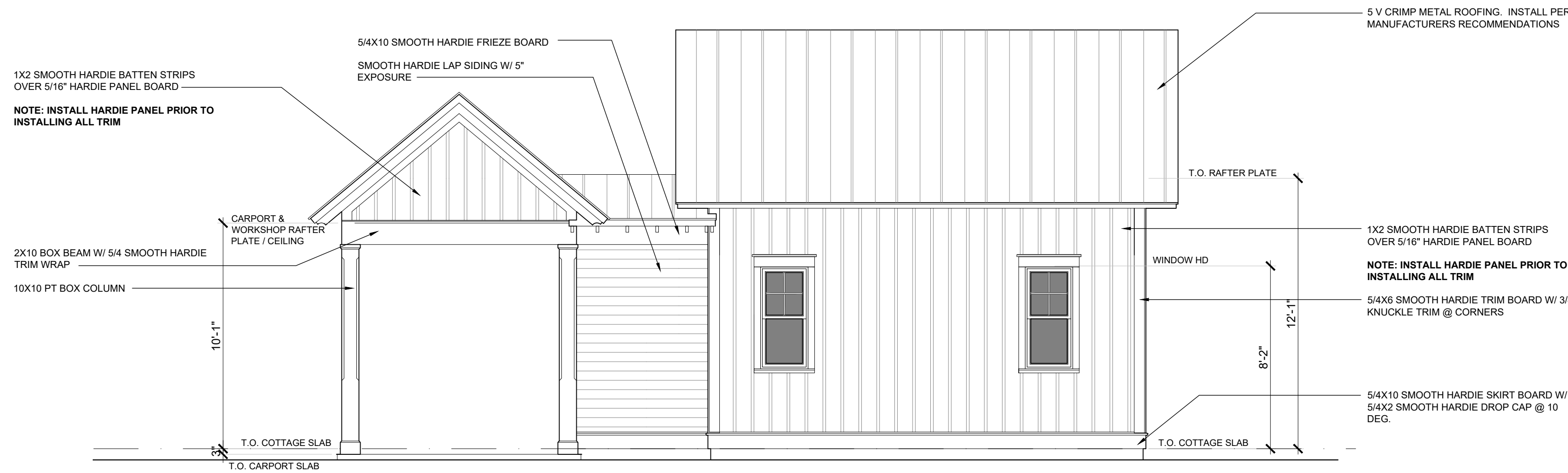
3 A3.0 REAR ELEVATION 1/4" = 1'-0" (SOUTH ELEVATION)
