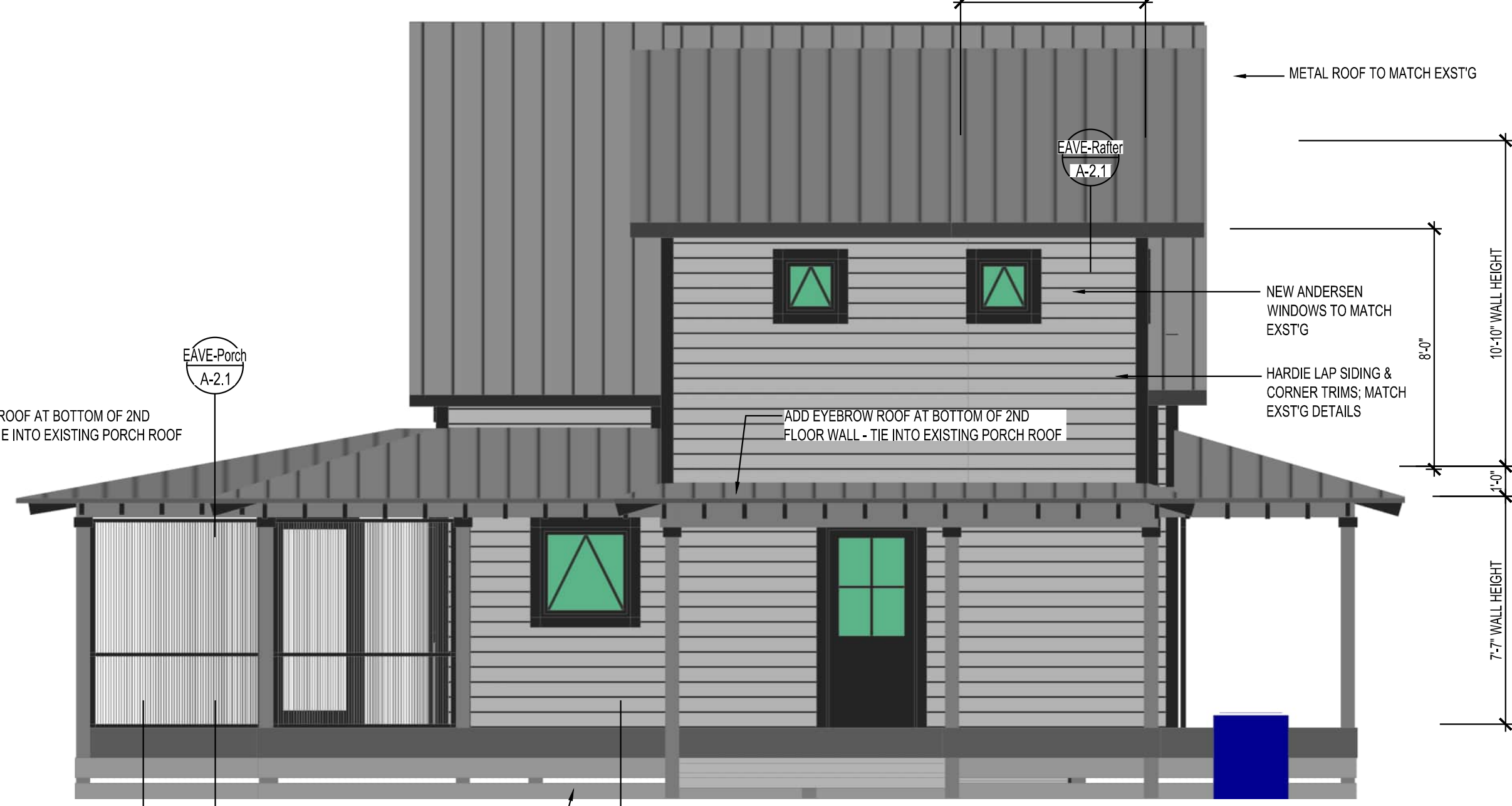
NEW NORTH ELEVATION 1/4"=1'
